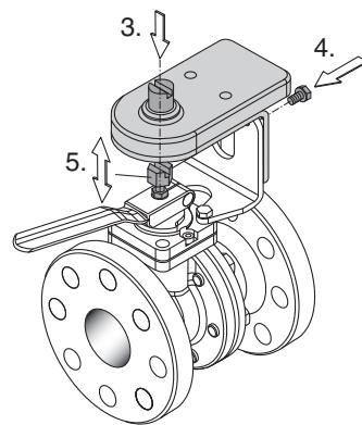
6. Install the actuator (puck) on top of the shaft and the valve sensor on the sensor plate.
