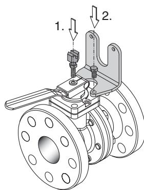
3. Attach the upper part of the mounting bracket with the sensor plate to the previously assembled base. The bore holes allow a rough height adjustment.
